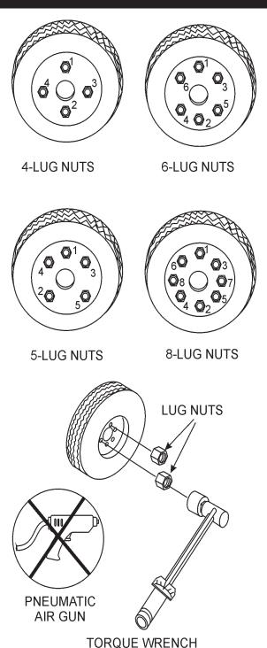
Figure 31. Wheel Lug Nuts Tightening Sequence
